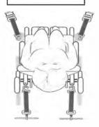
For hard-to-secure motorized scooters and wheelchairs, manufacturer's securement loops can be used. These loops, made from durable webbing, can be looped around the central drive shaft or seat frame and secured with two tie downs. Such straps can be permanently affixed to the mobility devices of frequent riders for easy securement.
